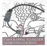
the shift again, continuing to dial out the adjuster as needed until the derailleur snaps crisply onto the cog. Progress up the cogs. When the shifting is perfect that way, repeat the routine coming down the cogset. This time if the derailleur hesitates, dial the barrel adjuster in just one-quarter of a turn at a time. You should be able to work your way up and down the cogset and fine-tune the shifting in less than 10 minutes.
