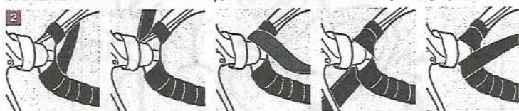
1 SPIRAL TAPE AWAY FROM BIKE AS YOU PASS OVER THE BAR
